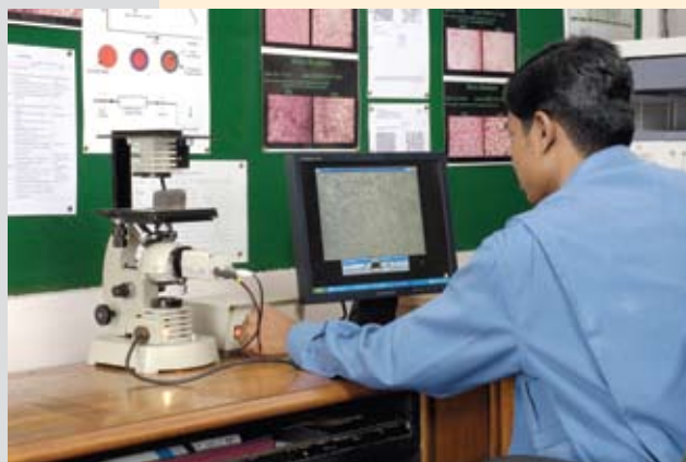
Micro Structure - Inverted stage metallurgical Microscope with digital CCD camera.
