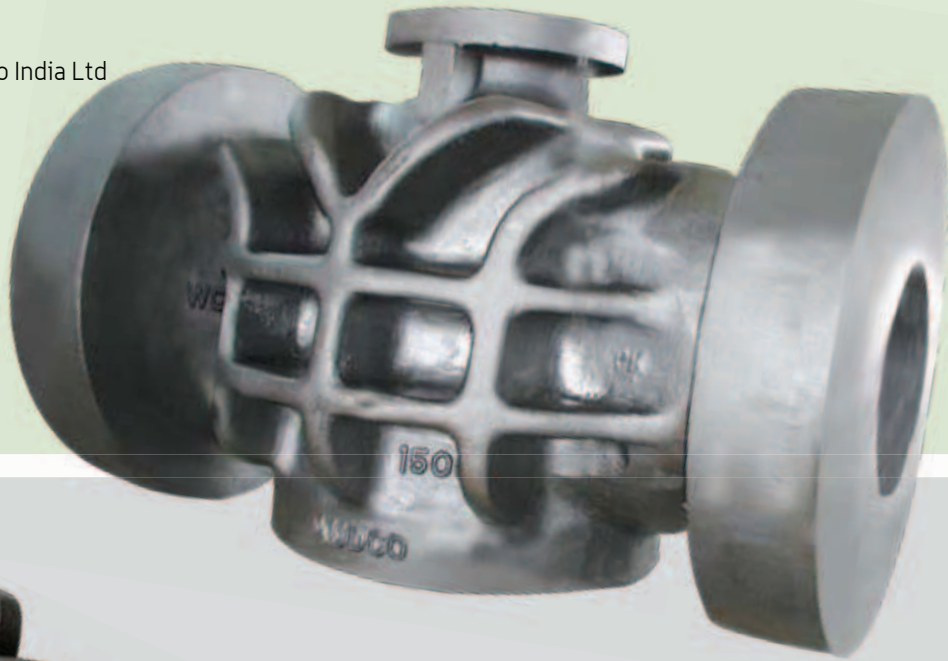
12" Cl. 1500 Body, Weight 3390 kg, Customer: M/s. Fisher Sanmar Ltd
