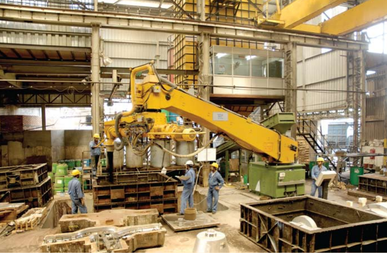
30 Ton IMF continuous mixer Alphasert process Heavy box moulding
