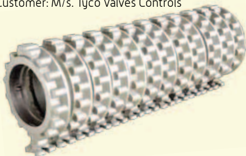
24" Fig 362 Lugged Bodies, Weight 258 kg, Customer: M/s. Tyco Valves Controls
