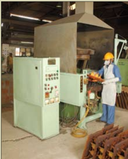
Shell moulding Matchplate Size: 600 x 450 x 250 mm
